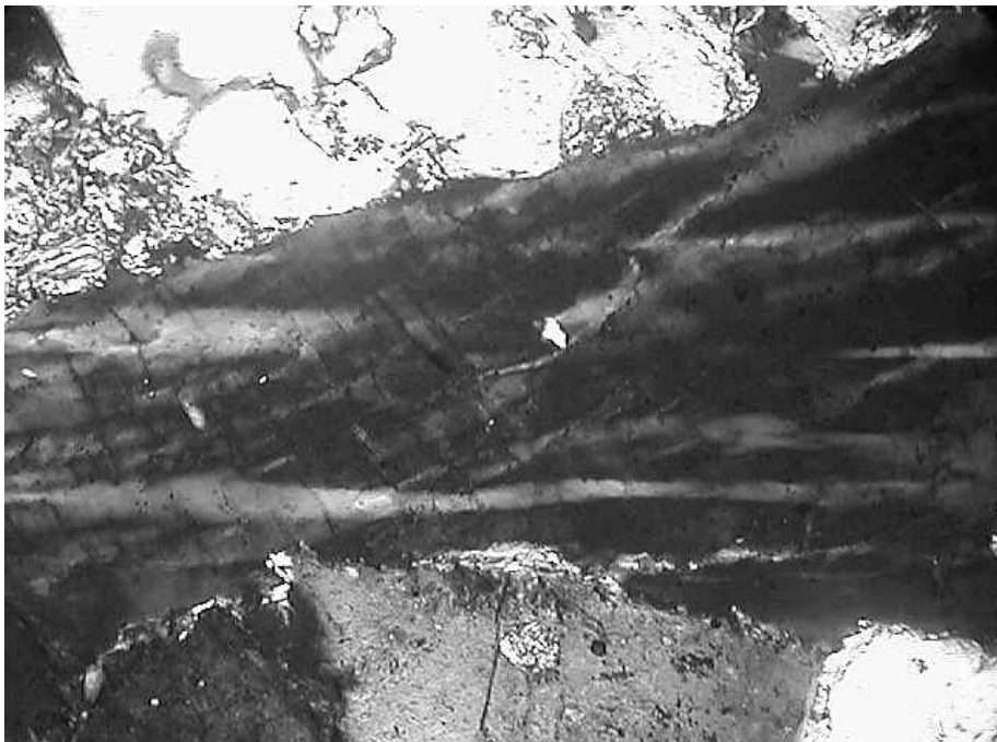
Multiple sets of kink banding in quartz and crossing planar features.
