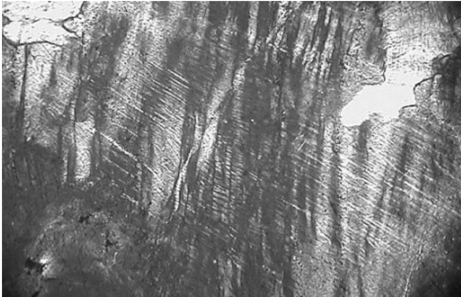
Deformation lamellae (N - S) and closely spaced kink banding (NW - SE).
