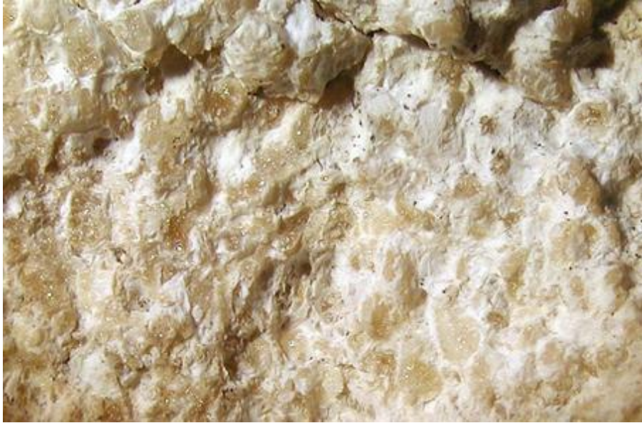
Carbonate-phosphate melt in close-up: Calcite amoebic bodies (darker) in a matrix of phosphate glass (white). The field is 30 mm wide.
