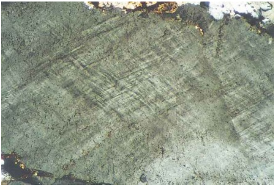
Multiple sets of planar deformation features (PDF) in quartz; shocked sandstone clast, Corbatón.
