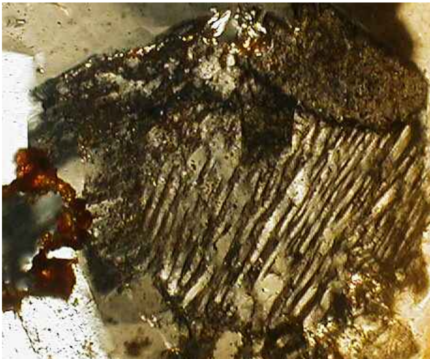
Shocked feldspar with isotropic (diaplectic) twin lamellae and faint PDF, XX. Sandstone, Buntsandstein central uplift in the 10 km-diameter Jiloca-Singra impact crater in the Jiloca "graben".
