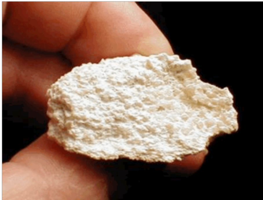
Carbonate-phosphate melt: surface of a break.
