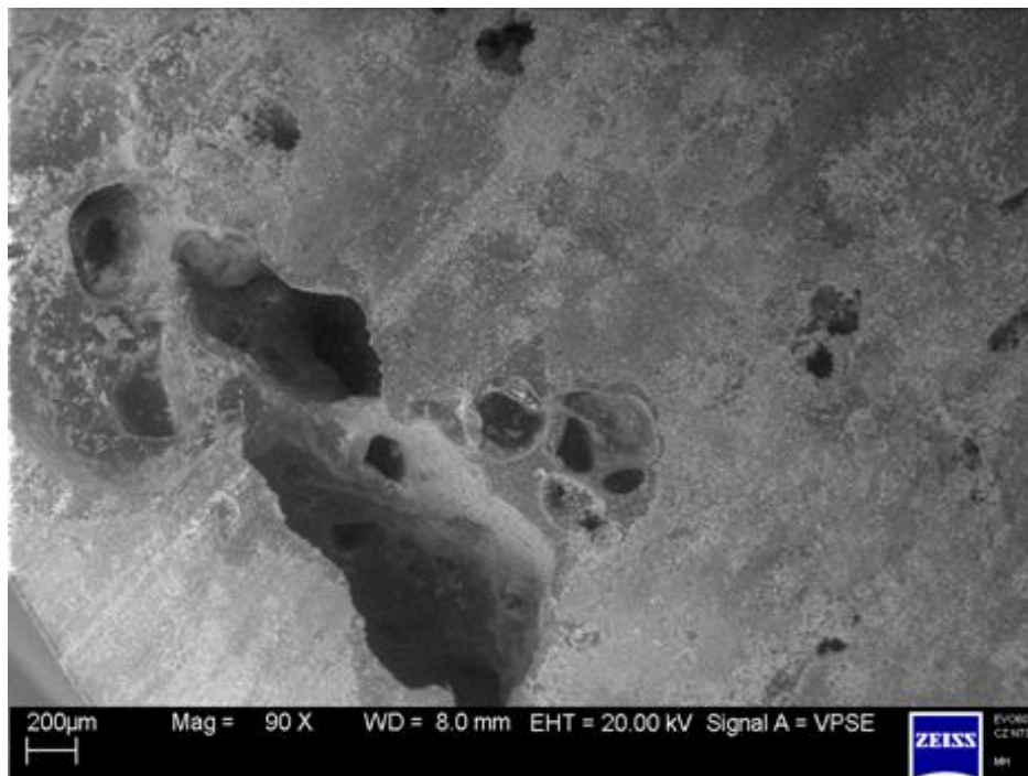
The sulfate melt rock under the SEM. Note the vesicular texture.
