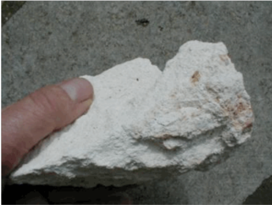
Carbonate melt rock from the Corbalán limestone quarry, southern impact basin. Close-up below.
