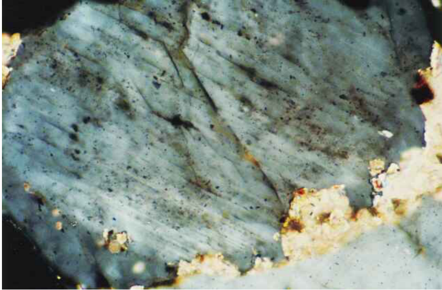
Planar deformation features (PDF) in quartz; shocked Cretaceous sandstone; Torrecilla ring near Portalrubio
