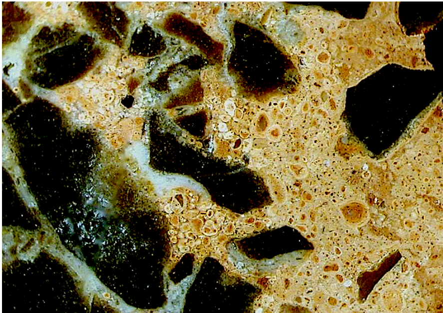
Close-up of the lapillistone matrix
