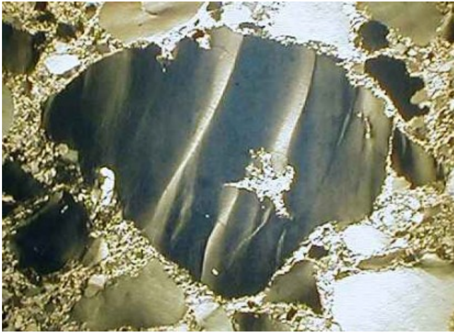
Plastically deformed kink bands in quartz and faint PDF.
