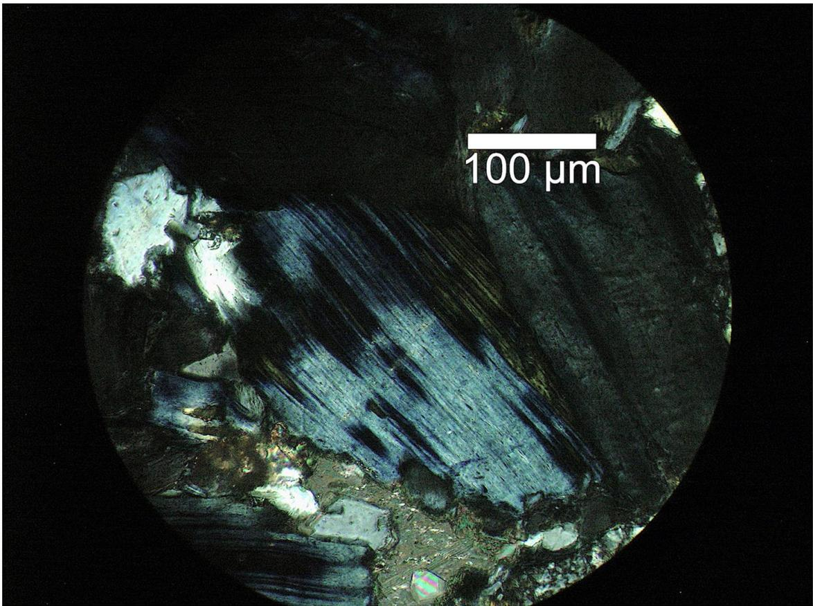
**Fig. 8. PDF merging into diaplectic glass in quartz.**
