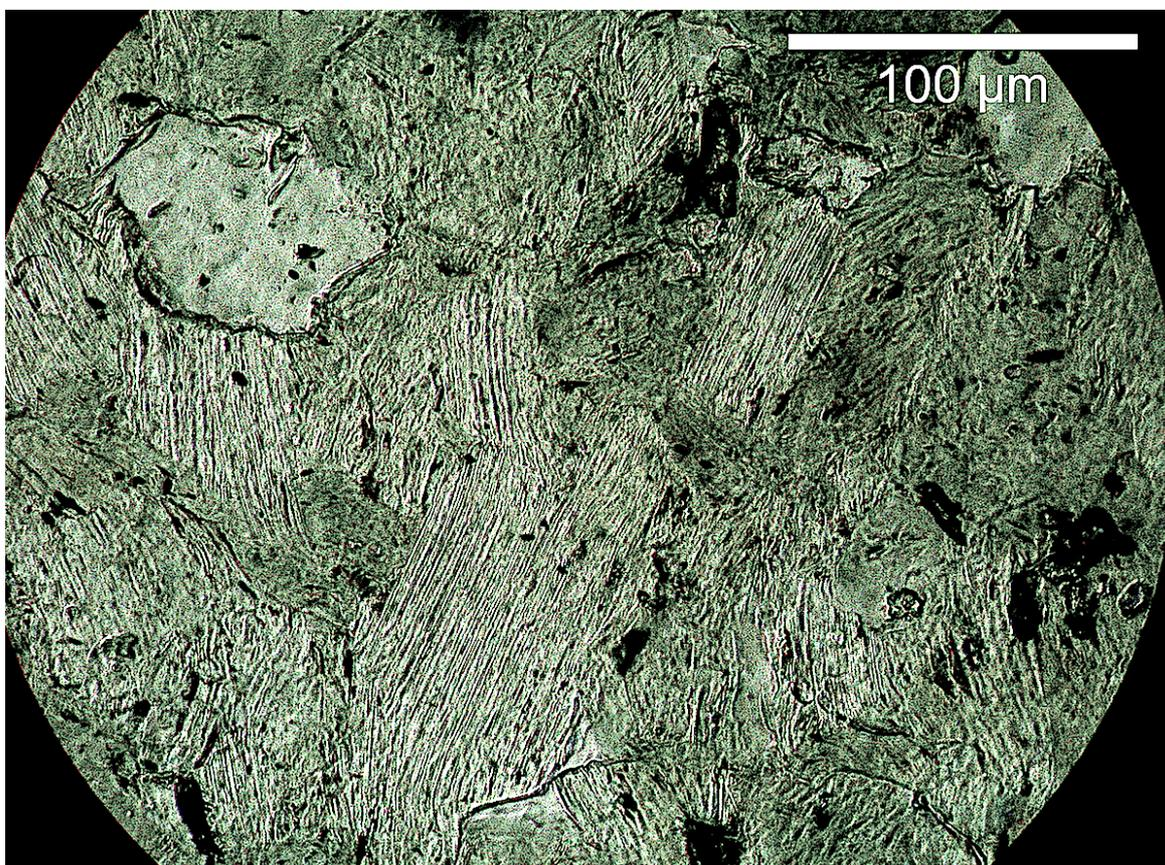
**Fig. 7. Densely formed PDF in quartz. Photomicro-graph, PPL.**
