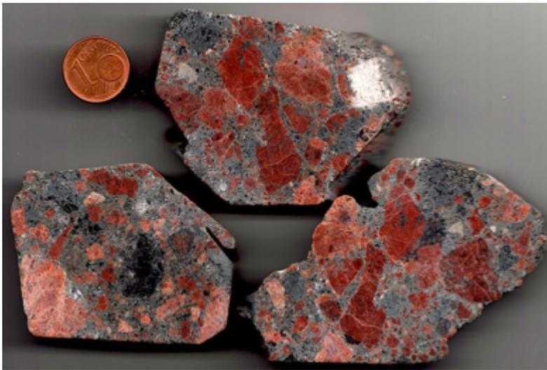
**Fig. 5. The so far most analyzed polymictic breccia from the outcrop. Breccias-within-breccia are common, and few three-generation breccias (breccia-within-breccia-within-breccia) are also observed.**
