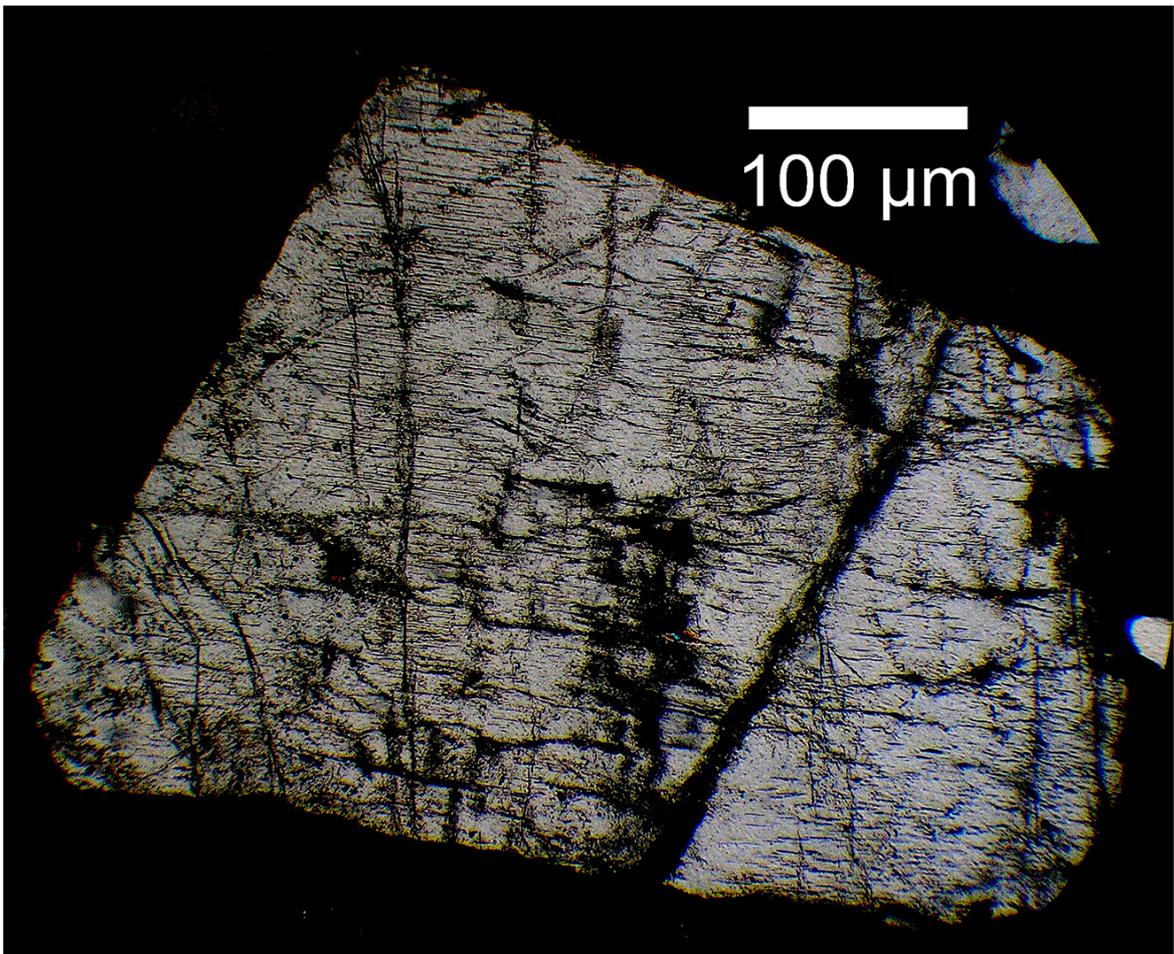
**Fig. 11.** The feldspar grain from Fig. 3 in higher magnification shows a pronounced set of PDF. A few more sets of different orientation are only faintly developed.
