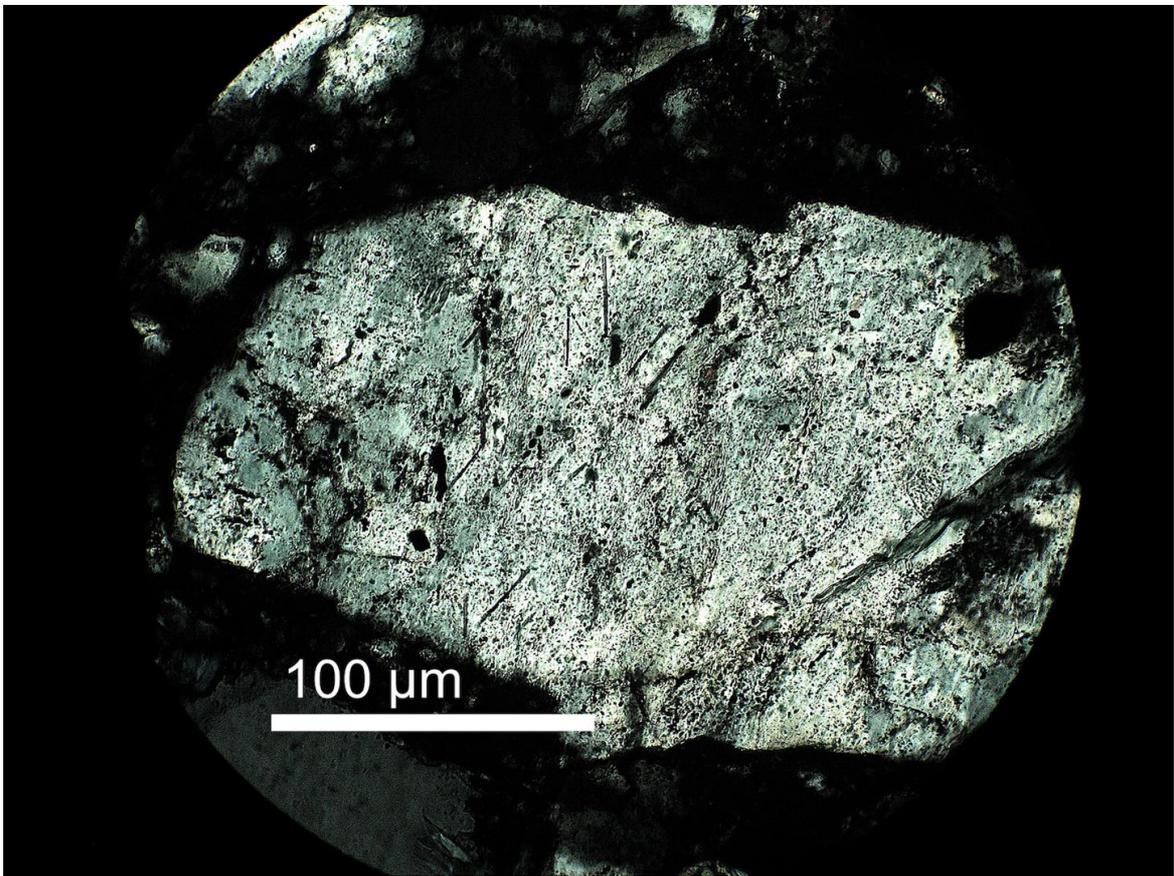
**Fig. 10.** Multiple sets of planar fractures (PF) in quartz.
