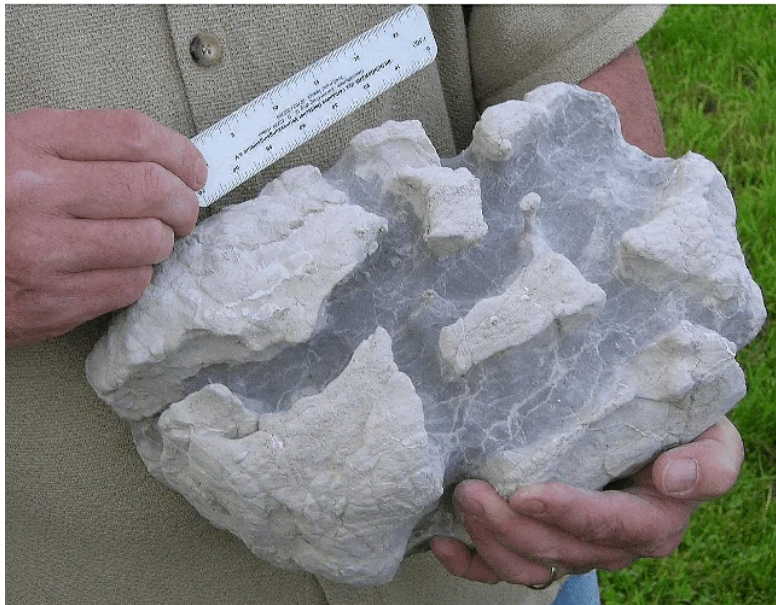
Impact corrosion by heat and/or nitric acid.
