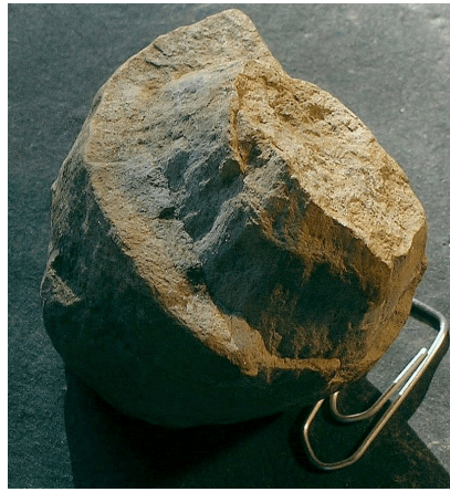
Shatter cones (counter cones) from the Lake Tüttensee crater rim proves impact shock deformation.
