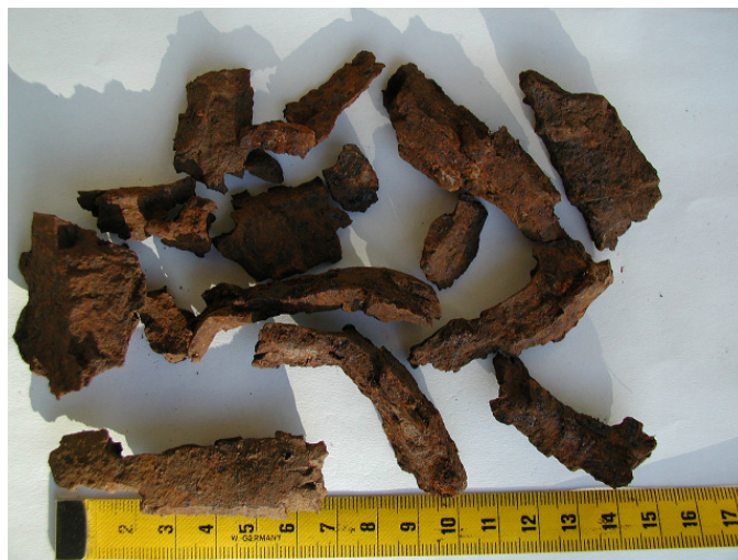
Fig. 2. Exploded ordnance iron splinters from the Sirente crater field. Photo W. Mayer.
