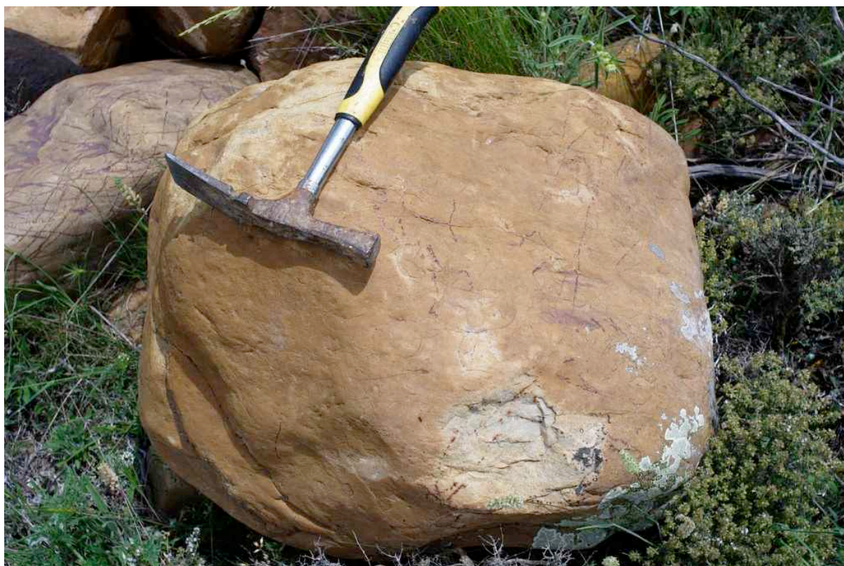
Fig. 15. Large quartzite block with distinct concussion marks. Close-up in Fig. 16.
