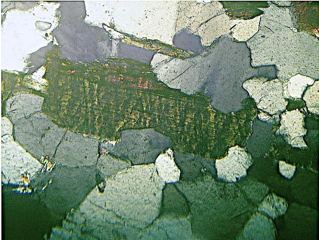
Fig. 42. Two sets of dense kink banding in biotite; gneiss. Crossed polarizers, field width 1 mm.
