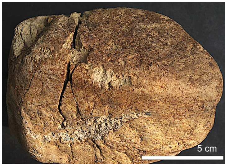
Fig. 48. Macroscopic impact shock spallation abundantly observed in the Chiemgau impact strewn field. Despite the widely open, only piecewise tensile fracture the quartzite cobble has remained coherent, which is also the case in the following examples.
