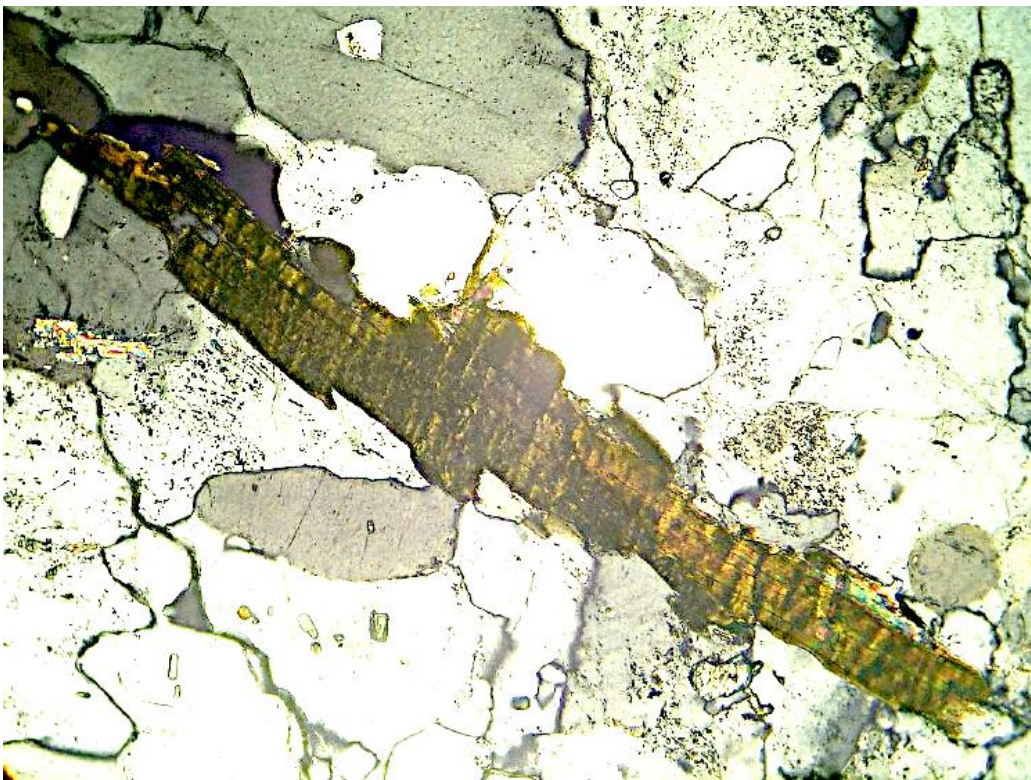
Fig. 43. Dense kink banding of slightly varying orientation in biotite; gneiss. The kink-band width is only 10 - 20 \mu\text{m} on average. Crossed polarizers, field width 1.4 mm.
